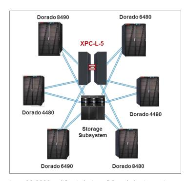
In an OS 2200 multihost cluster, all Dorado hosts must connect to each of two XPC-L-5 servers for total redundancy.
