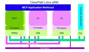
Multiple high-speed Ethernet connections are maintained within the PMM to provide MCP network connectivity.
